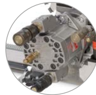
Main motor with leak-oil connection
