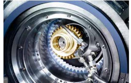
**+ System solution:** The design and specification of MIRA REX honing wheels are perfectly tailored for use with MIRA DDG diamond dressing gears.
