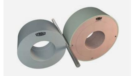
**+ Reduced wheel weight:** The innovative TYROLIT lightweight technology "N-LW" with a density 49% lower than aluminium greatly reduces the wheel weight compared to conventional grinding wheels. This protects the machine spindle, reduces the amount of energy required to drive the grinding wheel and reduces surface flaws.
